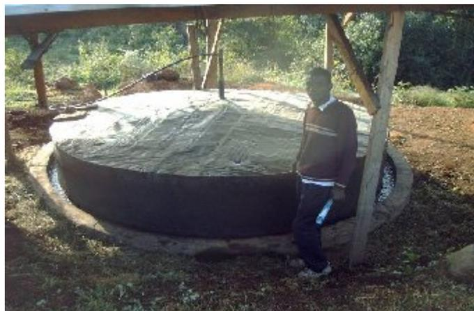
Figure 12. Inverted drum on digester raised by the presence of biogas
