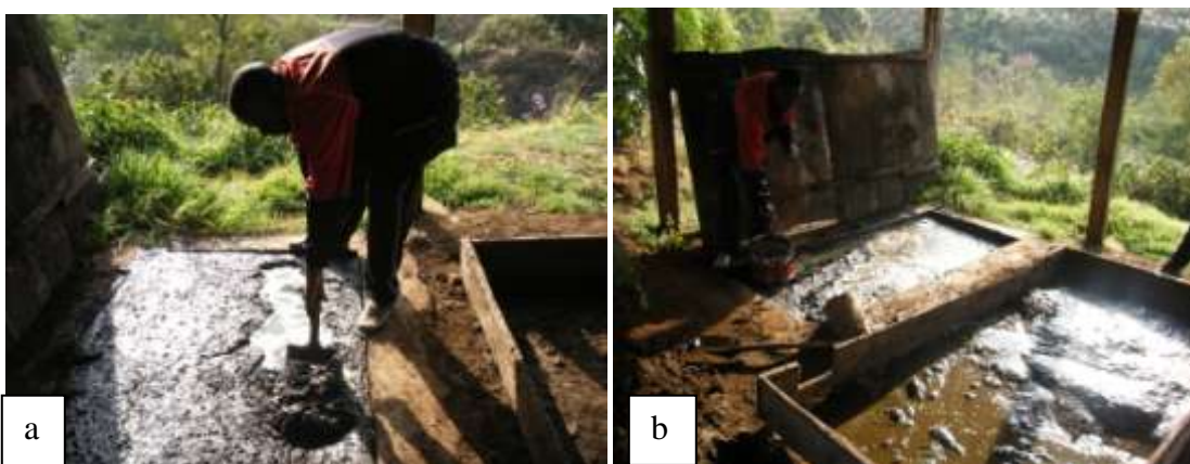
Fig.8. Obtaining pig dung for biogas production.a: BIOFARM piggery attached to the biogas system; b: biogas plant mixing tank.
