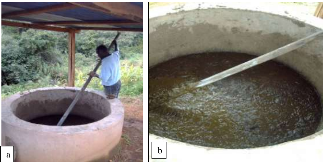
Fig. 2. Preparation of biogas slurry from pig dung and water. a : Biogas mixing tank; b : Fresh cow dung mixed with water to form slurry.
