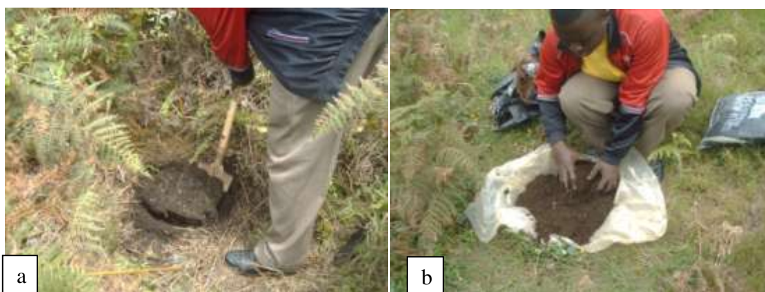
Fig. 7: Soil sample from research plot for analysis. a :Soil sample collection; b : Soil sample mixing.
